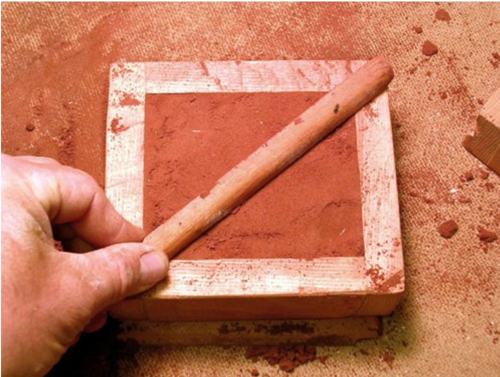
Scrape off excess sand.
